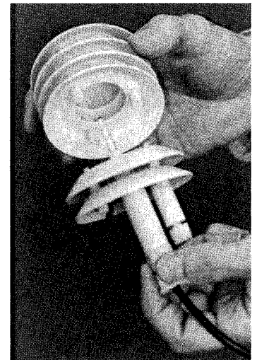
Two-part construction allows easy access for cleaning.
